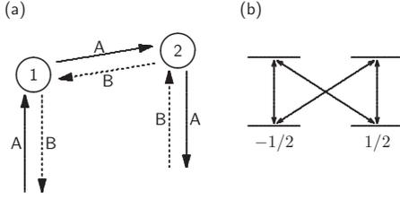
FIG. 1. (a) The two paths in coherent backscattering. Along path A the photon is first scattered by atom 1, then by atom 2; along path B the order is reversed. (b) Level scheme of the  $1/2 \leftrightarrow 1/2$  transition. Both the ground state and the excited state are doublets with total angular momentum  $j=1/2$ , and the magnetic quantum numbers  $m=\pm 1/2$  label the sublevels.
