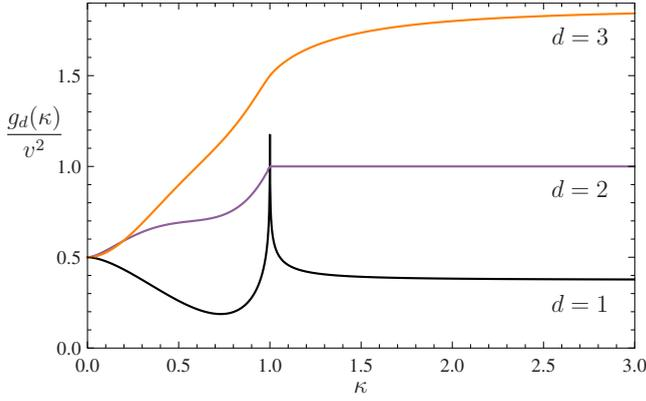
FIG. 5. (Color online) Correction to the density of states  $g_d(\kappa) = (\bar{\rho} - \rho_0)/\rho_0$  divided by the squared disorder strength  $v = V/\mu$  as function of reduced momentum  $\kappa = \omega\sigma/c$  in dimension  $d=1, 2, 3$ . At  $\kappa=1$ , the momentum beyond which elastic backscattering becomes impossible in the Born approximation, there is a logarithmic divergence in  $d=1$ , a kink in  $d=2$ , and a curvature discontinuity in  $d=3$ .
