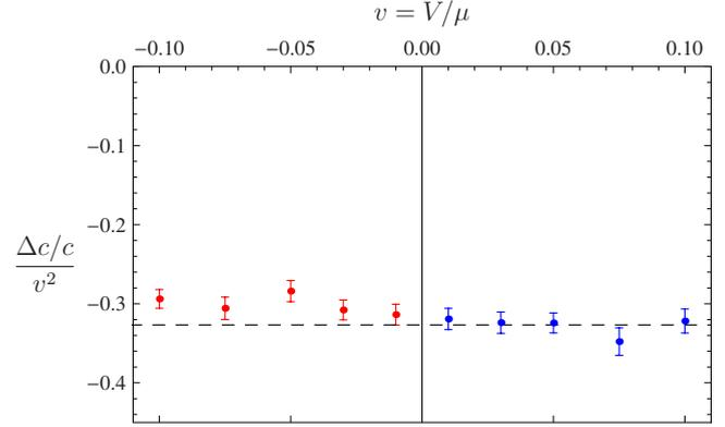
FIG. 3. (Color online) Relative correction to the speed of sound at  $k\sigma=1$ , divided by  $v^2$ , as function of disorder strength  $v=V/\mu$ , taken from the numerical integration with  $k\xi=0.05$ . (Dashed line) Analytical prediction  $\Delta c/(cv^2) = \frac{1}{4} \ln 2 - \frac{1}{2} \approx -0.3267$ .
